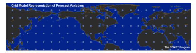
Derivatives are approximated at each grid point using a variety of arithmetic techniques called finite differences, as illustrated below. The choice of finite difference method affects both the computational error and amount of computer time required to run the model.
