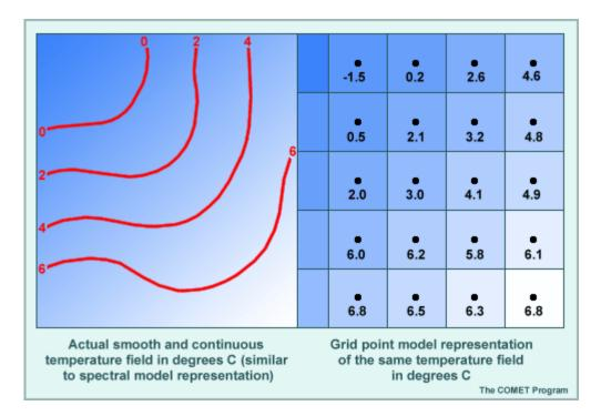
Grid point models, however, perform their calculations on a fixed array of spatially disconnected **grid points**. The values at the grid points actually represent an area average over a grid box. The continuous temperature field, therefore, must be represented at each grid point as shown by the black numbers in the right panel. The temperature value at the grid point represents the grid box volume average.
