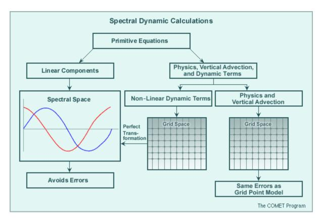
While vertical advections are calculated using finite differencing, which generates truncation errors, horizontal advections, including wind advection, are also calculated on grids. However, special mathematical properties avoid the introduction of error for these terms.
