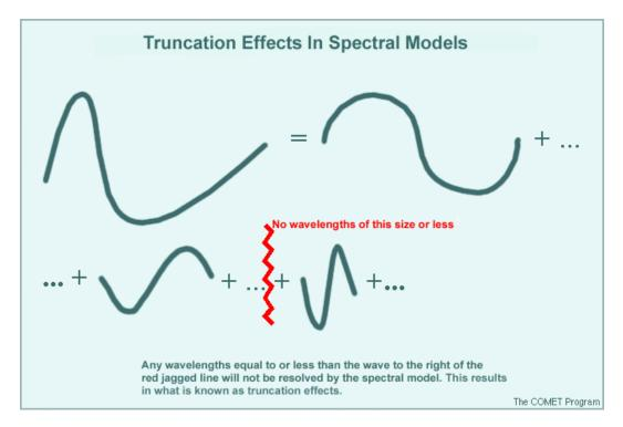
Several types of wave orientation are possible in spectral models. Triangular (T, as in T170) configuration is the most common in operational models since it has roughly the same resolution in the zonal and meridional directions around the globe.
