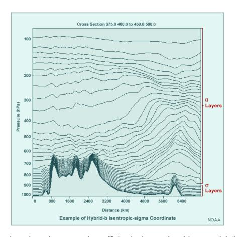
The boundary sigma layer must be sufficiently deep to be able to model diurnal boundary-layer processes, including friction and heating. This typically requires that the sigma boundary layer be approximately 200 hPa deep. If the sigma layer is too shallow, superadiabatic layers can still form or will not be treated properly above the boundary sigma domain.
