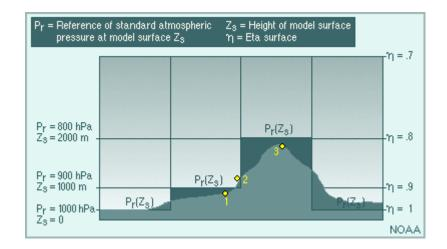
First, the heights at each model level must be defined. In this example, we have defined a model with 10 eta layers (only 3 shown) distributed evenly with respect to pressure from sea level to the top of the atmosphere. Standard atmosphere pressures are then determined at each of these heights.
