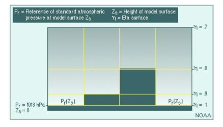
The eta coordinate is, in fact, another form of the sigma coordinate, but uses mean sea level pressure instead of surface pressure as a bottom reference level. As such, eta is defined as
