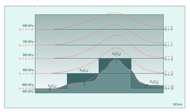
The fact that the eta coordinate is nearly horizontal and allows terrain features, such as mountains, to be depicted as blocks of solid earth in several levels of the model has several important advantages.
