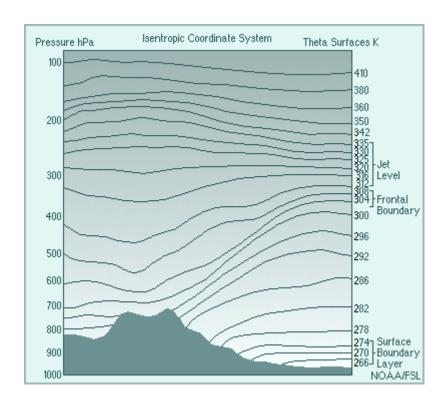
Since flow in the free atmosphere is predominantly isentropic, potential temperature (a) can be very useful as a vertical coordinate system. However, non-adiabatic processes dominate in the boundary layer and isentropic surfaces intersect the earth's surface. For these reasons, potential temperature alone is not currently used as a vertical coordinate in any operational numerical model system. However, isentropic coordinates do form an essential part of many hybrid vertical coordinate systems.
