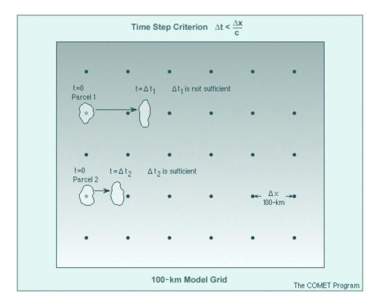
Let's look at an example of a hypothetical model with a Ax of 100 km. You might assume that a time step of an hour or so would be sufficient to forecast synoptic-scale motions. However, the model generates waves with propagating speeds in excess of 100 m/s relative to the winds, which themselves may reach 100 m/s in the jet core. So we need to consider the wave speed of the fastest wave in the model, at least 200 m/s. Using this value for c yields the following:
