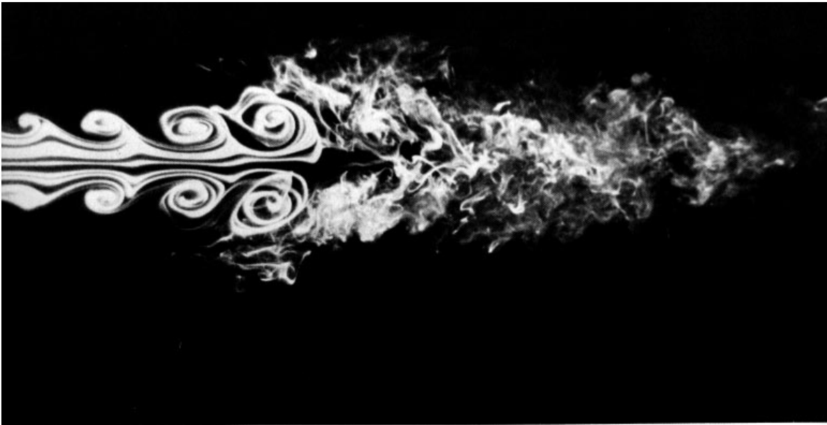
102. Instability of an axisymmetric jet. A laminar stream of air flows from a circular tube at Reynolds number 10,000 and is made visible by a smoke wire. The
