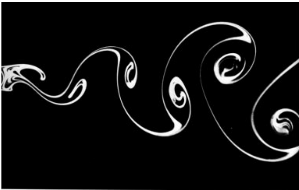
94. Kármán vortex street behind a circular cylinder at \text{Re}=140 . Water is flowing at 1.6 \text{ cm/s} past a cylinder of diameter 1 cm. Integrated streaklines are shown by electrolytic precipitation of a white colloidal smoke, illuminated
